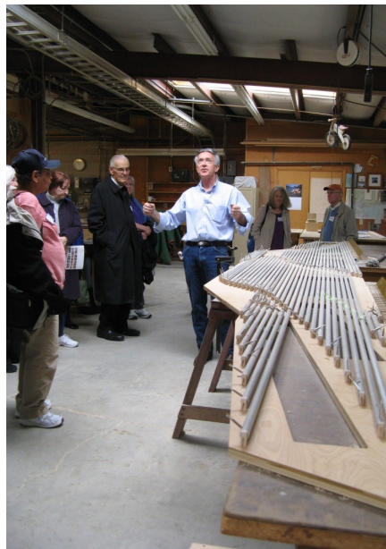
that are cut and rolled into pipes. All are assembled & tested before shipping.—Photos by Frances Nilsson.
